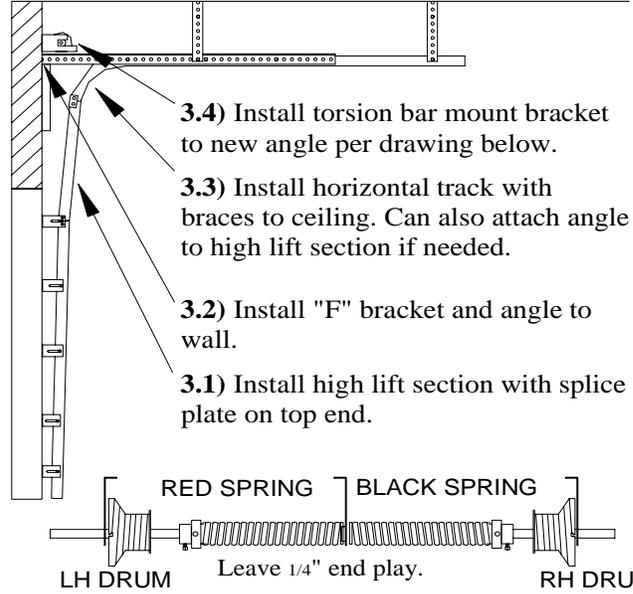
3.4) Install torsion bar mount bracket to new angle per drawing below.
